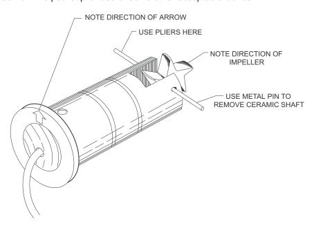
10. Install the sensor into the 2 inch NPT adapter or tee so that alignment hole is facing upstream and flow arrows point in the direction of the actual flow. Since the positioning collar was not loosened during this operation,
